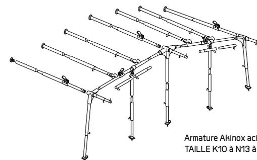
Armature Akinox acier Ø25 mm
